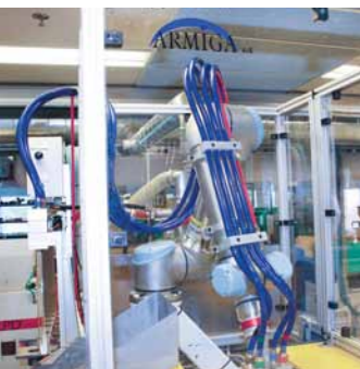
Oticon also uses the robot for a different task in the foundry where the suction tool is replaced with a pneumatic gripping tool used for handling more complex cast parts. The robot works in cycles of 4-7 seconds.
