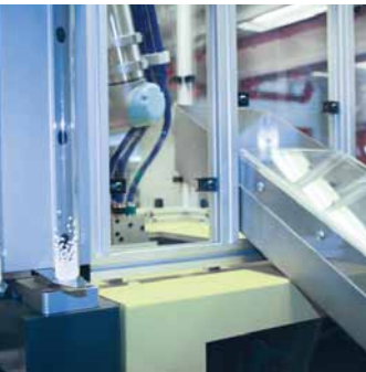
The robot is securely fitted to the injection moulding machine and can move over the mould and pull up the plastic items. This is done using a specially designed vacuum system which ensures that the sensitive items are not damaged.
