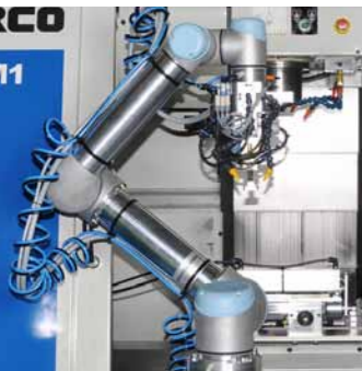
The robot opens both doors, puts in the raw material, tightens the machine's vice, removes it again after milling and puts it to one side.
